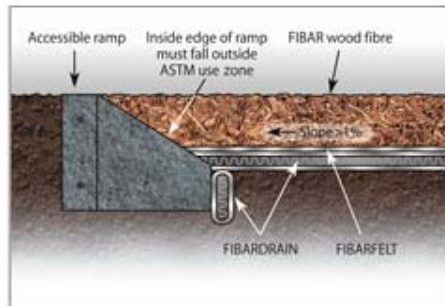
Figure 5. Entrance and exit ramps into the Fibar surface should have a minimum slope of 1 in 12 or must meet current ADA, state or local regulations.
